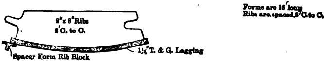
PLATE 156.—Details of Wooden Form Used for 2-in. Mortar Lining for Steel Pipe Siphons. As improved on Contract 68.
